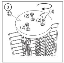
(3) Use hammer or mallet and gently hammer in plastic screw about 1/8" down onto threaded end of wire.
